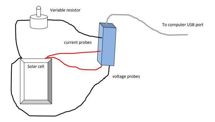
4) Open the DataStudio activity called JVcurve.ds. It will display a graph with amps on the y axis and volts on the x, and a dial display for current and voltage meters. The sampling option is set to "Manual Sampling" and "Keep data values only when commanded. On both meters and graph the appropriate range is 0-.1 amps for current and 0-.5 volts.
